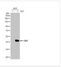
Western Blot: OAT Antibody (HL2087) - Azide and BSA Free [NBP3-25584] - Various whole cell extracts (30 ug) were separated by 10% SDS-PAGE, and the membrane was blotted with OAT antibody [HL2087] (NBP3-25584) diluted at 1:1000. The HRP-conjugated anti-rabbit IgG antibody was used to detect the primary antibody, and the signal was developed with Trident ECL plus-Enhanced.
