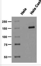
Simple Western: CRISPR-Cas9 Antibody (6G12) - C-terminus - Azide and BSA Free [NBP2-80680] - Image shows a specific band for Cas9 in 0.2 mg/mL of HeLa Cas9 lysate but not in Hela WT lysate. This experiment was performed under reducing conditions using the 12-230 kDa separation system. Observed molecular weight is ~158 kDa. Image from the standard format of this antibody.
