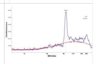
Simple Western: c-Myc Antibody (9E10.3) [NBP2-45144] - Lane view shows a specific band for c-Myc in 0.2 mg/mL of HeLa lysate and antibody at 20 ug/mL. Electropherogram image of corresponding Simple Western lane view at WES molecular weight of 74 kDa. Image reported by internal validation.
