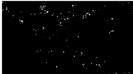
(E) Remove background with a blank image match distance = 2, multiplication factor = 1.1 (optimal)
