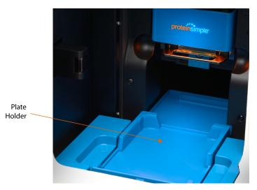
Sample plates should be inserted into the plate holder so that the A1 well position is aligned with the upper left corner of the tray.
