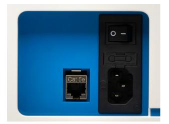
System Power - The main system power components consist of the power switch and power input.
