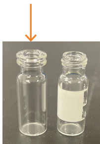
MauriceFlex glass crimp top reagent vial (PN 110-0019, left) and glass reagent vial (PN 046-017, right) Only MauriceFlex glass crimp top reagent vials (PN 110-0019) should be used to prepare MauriceFlex cIEF batch reagents.
