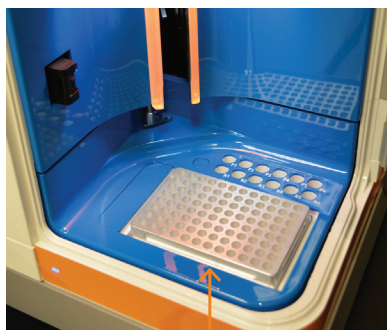
96-well Plate Insert for Maurice, Maurice C. and Maurice S.
