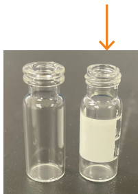
MauriceFlex crimp top glass vial (PN 110-0019, left) and glass reagent vial (PN 046-017, right) Only glass reagent vials (PN 046-017) should be used to prepare cIEF batch reagents.
