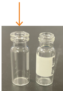
MauriceFlex glass crimp top reagent vial (PN 110-0019, left) and glass reagent vial (PN 046-017, right) Only MauriceFlex glass crimp top reagent vials (PN 110-0019) should be used to prepare MauriceFlex Fractionation batch reagents.
