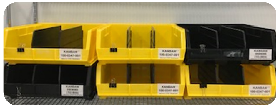
Reusable Bin Kan Ban System
