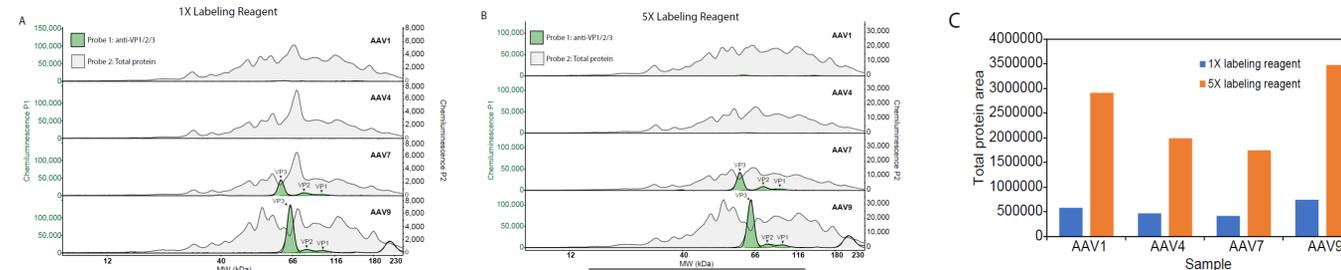
Figure 3. Evaluating 5X total protein in RePlex of AAV in-process samples. AAVs (1x10<sup>9</sup> GC/mL) were diluted 1:20 and analyzed on Jess using an anti-VP1/2/3 antibody (Progen) followed by RePlex with the (A) 1X or (B) 5X total protein. (C) Total protein area for each AAV sample were quantified.
