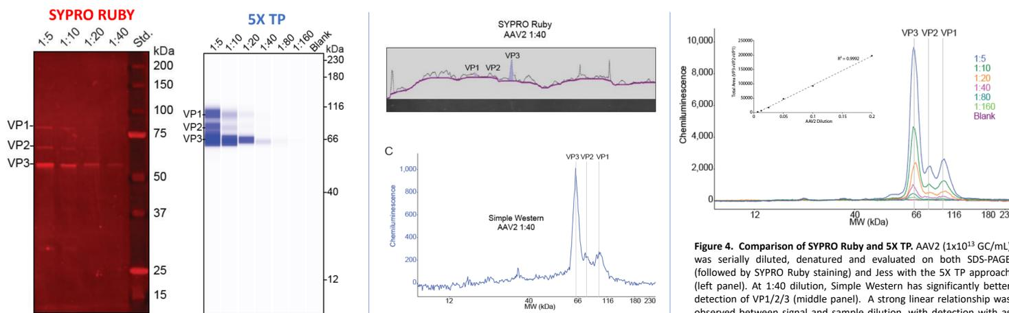
Figure 4. Comparison of SYPRO Ruby and 5X TP. AAV2 (1x10<sup>13</sup> GC/mL) was serially diluted, denatured and evaluated on both SDS-PAGE (followed by SYPRO Ruby staining) and Jess with the 5X TP approach (left panel). At 1:40 dilution, Simple Western has significantly better detection of VP1/2/3 (middle panel). A strong linear relationship was observed between signal and sample dilution, with detection with as little as 1:160 diluted AAV2 (right panel).
