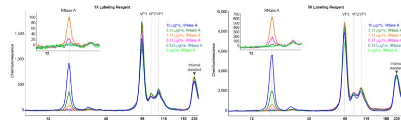
Figure 2. Recombinant RNase A impurity model in pure AAV2. AAV2 was spiked with RNase A (10, 3.33, 1.11, 0.37, 0.123 and 0 µg/mL) and prepared in 1X MM and denatured under reducing conditions for 10 minutes at 70 °C. Samples were then loaded onto a Jess and run with either 1X (left) or 5X total protein (right).
