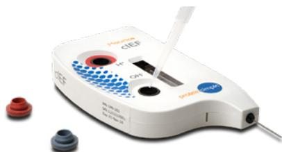
5. Seal each tank with the rubber stoppers. Use the grey stopper for the OH<sup>-</sup> tank and the red one for the H<sup>+</sup> tank. If excess liquid comes out of the tank, make sure to wipe it with a lint-free laboratory wipe.
