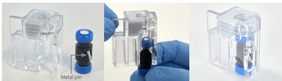
Figure 1. Assembling the Top Running Buffer vial in the cartridge insert.
