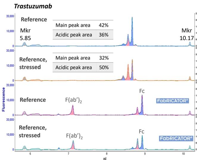
**Figure 3.** Trastuzumab was analyzed with Maurice icIEF for charge heterogeneity. In the stressed sample (7d at 37°C), there is an increase in the acidic peak area compared to the control. Digesting with FabRICATOR leads to the generation of F(ab')<sub>2</sub> and Fc fragments and allows to pinpoint the increase in acidic variants to the Fc region while the Fab remains largely unchanged.
