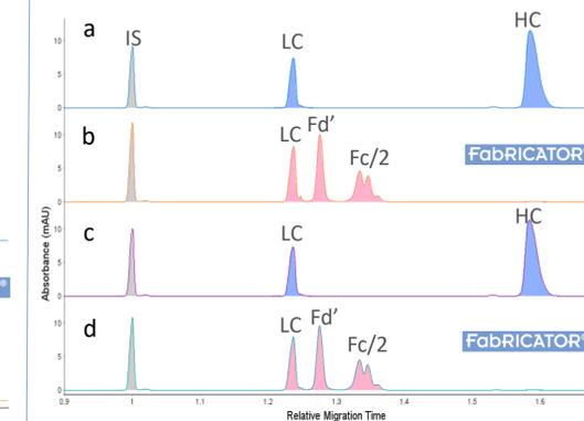
**Figure 6.** Relative migration time of Trastuzumab fragments after reduction (a) or treatment with FabRICATOR followed by reduction (b). A stressed sample of trastuzumab (7d at 37°C) was analyzed in the same way (c and d).
