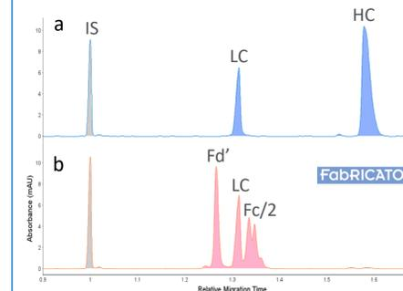
**Figure 5.** USP129 mAb was analyzed after reduction (a) or treated with FabRICATOR and then reduced (b). This subsequent reduction results in the separation of the F(ab')<sub>2</sub> fragment into smaller LC and Fd' subunits.
