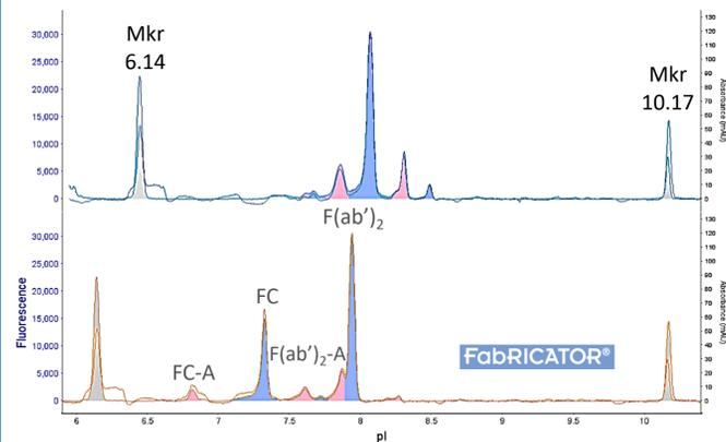
**Figure 2.** USP129 reference standard, monoclonal IgG, was treated with FabRICATOR, a cysteine protease that targets a specific sequence of IgG below the hinge region producing F(ab')<sub>2</sub> and Fc fragments. This treatment allows for localization of the charge variants to the different domain of the antibody.
