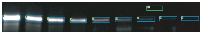
Figure 12. Standard Curve Calculation. In this example regions 1-9 were selected and the known concentration of each band was entered.
