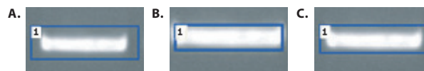
Figure 3. Demonstration the proper technique for drawing a region of interest around an object. A. Region too large B. Region too close to band C. Recommended Region placement.
