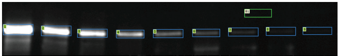
Figure 16. Standard Curve Calculation. In this example regions 1-9 were selected and the known concentration of each band was entered.
