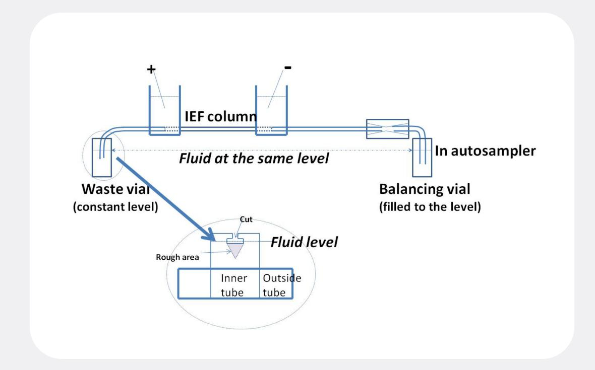
As shown in the above figure, the waste vial has a special cut at the top of its inner tube. Combined with the rough area beneath the cut, this structure ensures that the fluid inside the inner tube flows into the outside tube at a fixed level when the inner tube is filled higher than this fixed level (as indicated in the figure). The actual fluid level in this waste vial is within  $\pm 1$  mm of the designed level.
