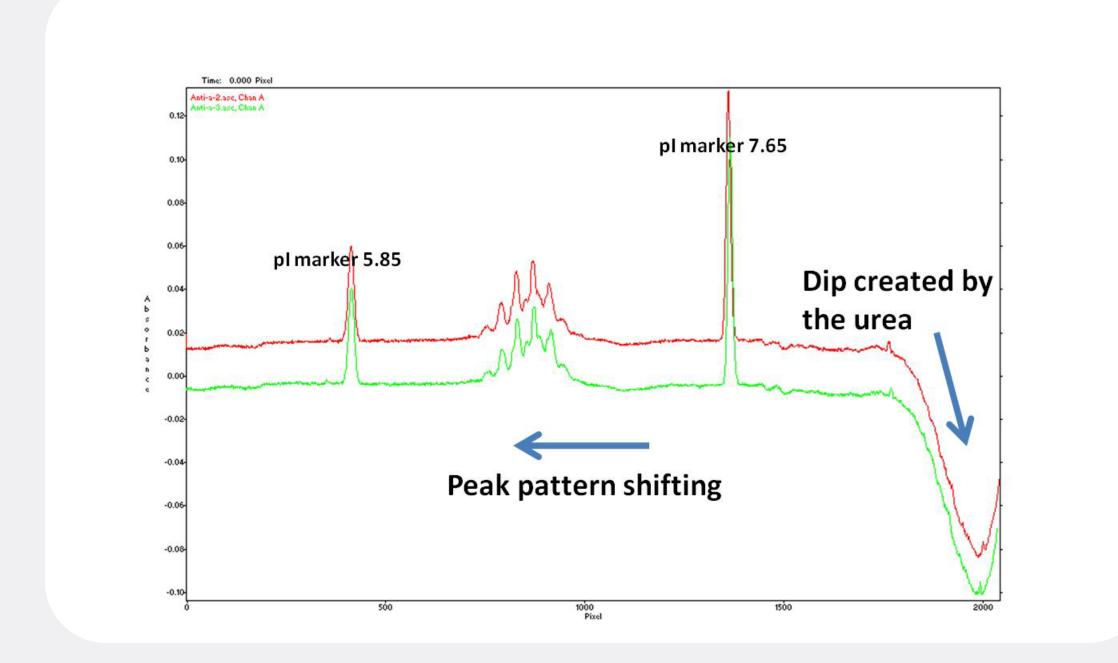
The dip observed in the above figure is caused by urea. Since urea has weak absorption at 280 nm (iCE's detection wavelength) during the IEF process, when the peak pattern shifts, electrolytes in the two electrolyte tanks at both ends of the capillary column may invade the column. The electrolytes have no absorption at 280 nm, thus creating a dip in the baseline.
