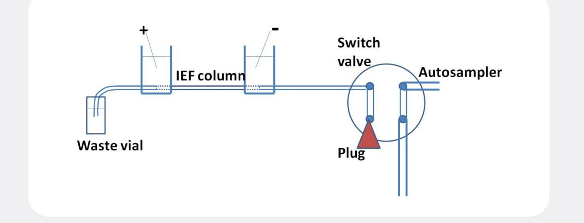
In the above configuration, the sample can be injected from the autosampler into the IEF column when the column is connected to the autosampler. During the IEF process, the switch valve turns to another position cutting off the connection between the column and the rest of the plumbing system.
