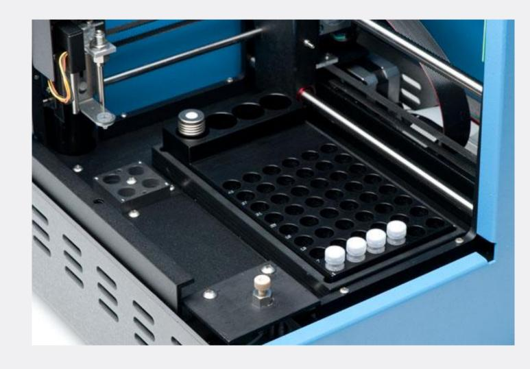
As shown in the previous picture, the sample tray can hold forty eight 1.5-mL sample vials or in the 96-well microplate version, 96 sample wells. The big vial positions in the back of the tray can hold up to three10-mL IEF buffer vials. The buffer vials are also cooled in the tray.
