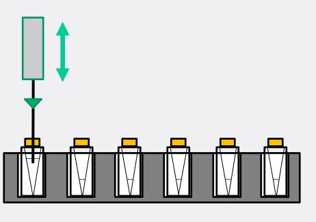
The dumped buffers are mixed with protein sample solution in the sample vial by the autosampler needles. In each mixing stroke, the needle aspirates 70% of the total solution in the vial and dumps the solution back into the vial while the needle moves up and down to mix the solution in the vial.
