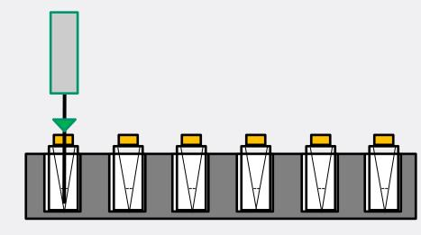
Just prior to injection of a sample in the sample tray, the autosampler needle aspirates the IEF buffers stored in the 10-mL vials and dumps the buffers into the bottom of the sample vial.
