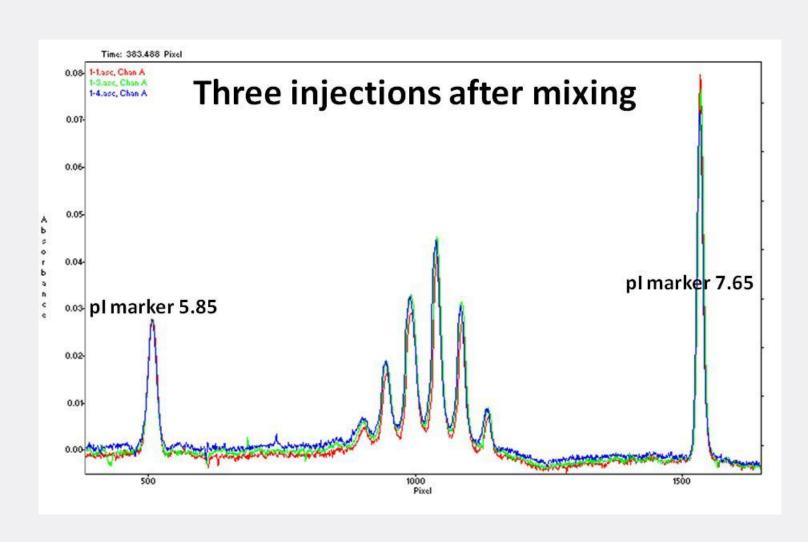
The figure above shows results of three consecutive injections from a sample vial after the sample is prepared by the autosampler. The protein sample is a monoclonal antibody and is mixed with 1% Pharmalytes 3-10, 3% Pharmalytes 5-8, 0.35% methylcellulose, 4 M urea and two pl markers.
