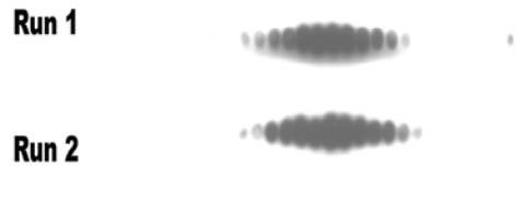
Figure 3: Reproducibility of dPC™ Western Analysis. 0.05 µg biotinylated ovalbumin was fractionated on pH 4.20 to 6.20 dPC™. The ovalbumin was transferred to PVDF membrane using the tank method. After blocking, the blot was probed with HRP-streptavidin and ECL substrate.
