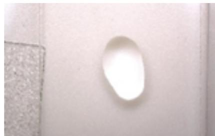
**FIGURE 2.** Water bead test failure, indicating a degraded silane coating.
