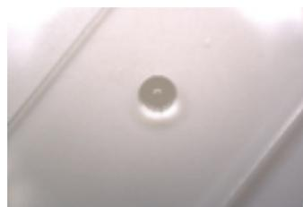
**FIGURE 1.** A 5  $\mu\text{L}$  water bead on the glass surface of a flow cell at  $t = 0$ , showing the intact silane coating.
