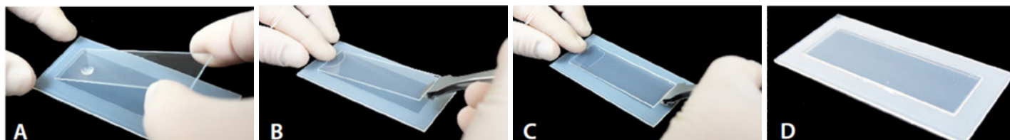
FIGURE 1. Original probing protocol recommended for use with a standard (full-chip) antibody probing chamber. A) Pipette antibody cocktail solution in a bead on the left side of the incubation fixture. B) Gently lower the chip onto the antibody cocktail. C) Stabilize the scWest chip gel side down using the flat edge of tweezers (without gripping with the tweezers). D) scWest chip incubating in antibody cocktail solution with no air bubbles.
