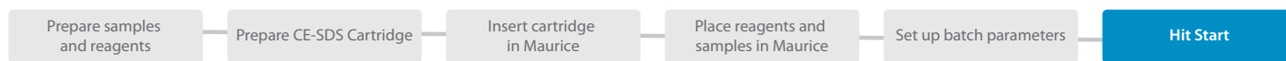
FIGURE 3. CE-SDS Workflow using Maurice. It takes less than 10 minutes to start a run once your samples and reagents are prepared.
