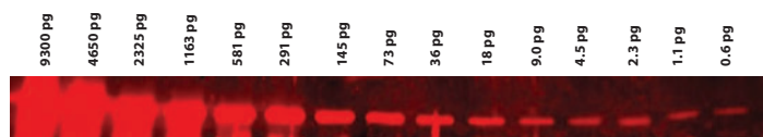
Figure 3. A lower limit of detection of 0.6 pg Transferrin was achieved with a 256 second exposure time.
