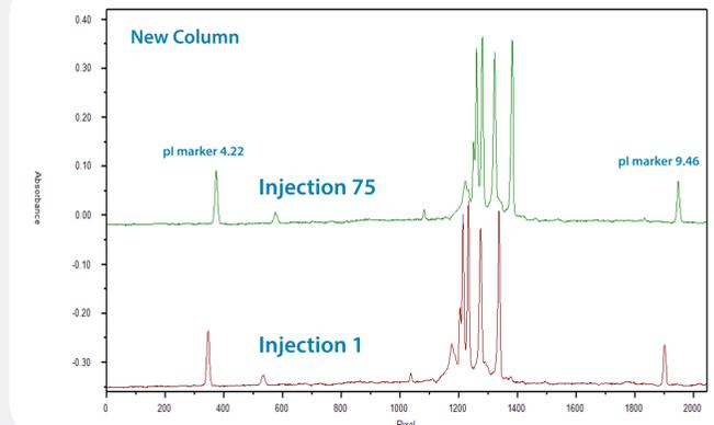
Figure 5: A compare plot of the first and 75<sup>th</sup> injection on the new column.
