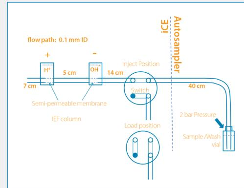
Figure 1: Flow path of the iCE IEF Analyzer.
